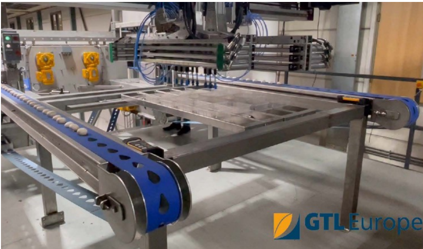
Sorting and packing robot with belt for moving picked mushrooms
