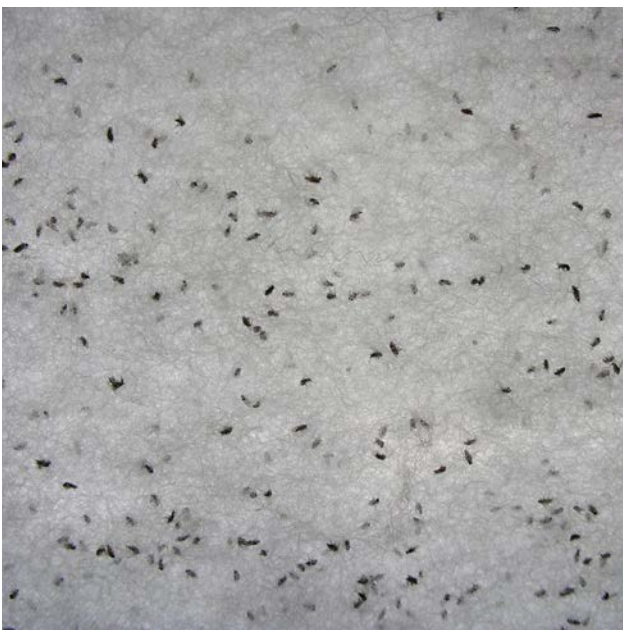
Figure 5. Flies can penetrate some washable fibrous pre-filter material. Image: J Allan
