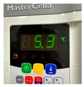
Check the calibration of your cold room using an accurate data logger or thermometer.
