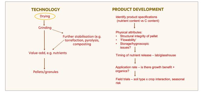
Steps required in SMS value adding, with drying representing a key limiting step in the development of pellets or granules. Adapted from Wilkinson et al, 2023, webinar presentation
